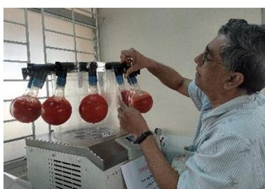
Fig.2. Extraction of annatto powder using freeze dryer
